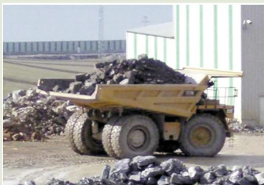
Figura 13. 4. Dúmper transportando material
